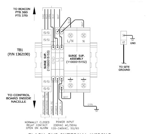
FLASH OVP INTERNAL WIRING
