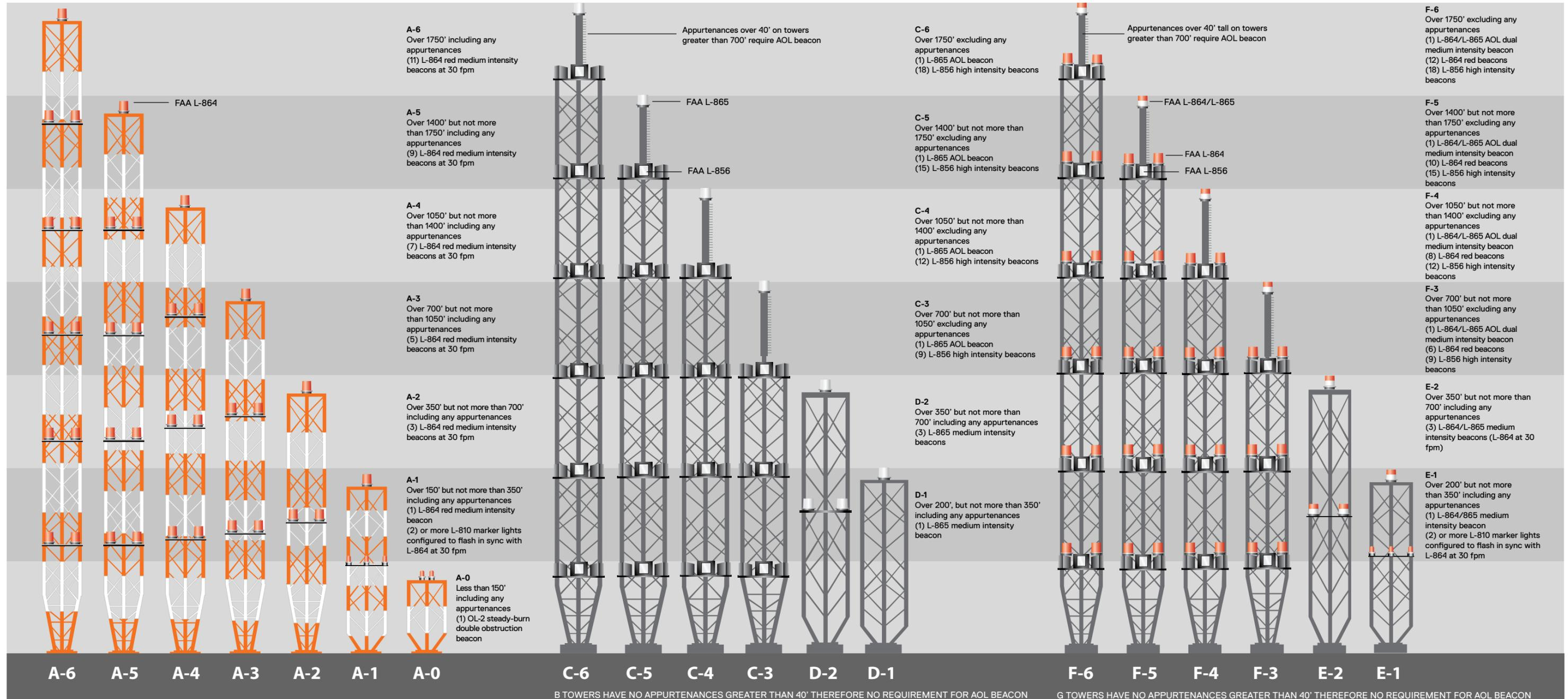
These guidelines are for reference only and are not to scale. FPM means flashes per minute. Please contact Flash Technology or the Federal Aviation Administration for specific questions regarding obstruction marking. All heights are based on AGL (above ground level) measurements.
