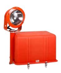
The FTS 830 is a current-driven unidirectional approach light that identifies runway end or the acquisition of an active runway. It can be used as a simple runway end identifier lights (REIL) or as an addition to complete any number of approach light systems like MALSR, MALSF, SSALSR, ALSF I and II for runway alignment and runway threshold marking.
